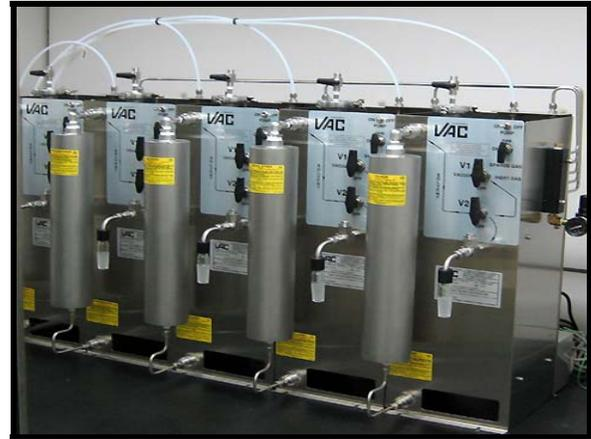
**Utilities Required:** The unit requires high-purity inert gas and a solvent resistant vacuum source for operation. See Options on page 3.
